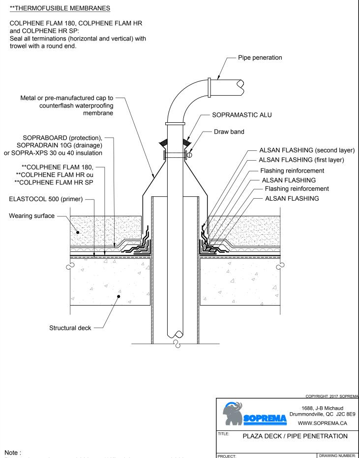
Penetrations to be spaced 300 mm (12") minimum apart and 300 mm (12") minimum from walls and curbs.
